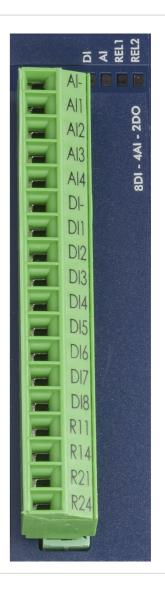
(\*) Terminal numbers R11, R14, R22 and R24 are derived from 11 (Common) and 14 (NO) that refer to the Single Pole, Single Throw, Normally Open (SPST NO) relay terminal numbering as per standard EN 50005.
